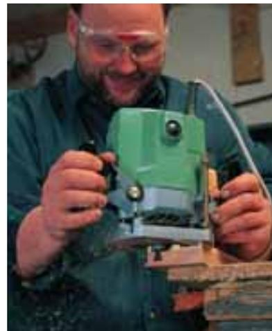
**4** Here you can see how the bushing rides against the template, while the bit cuts the pins. When you cut your pins be sure to
