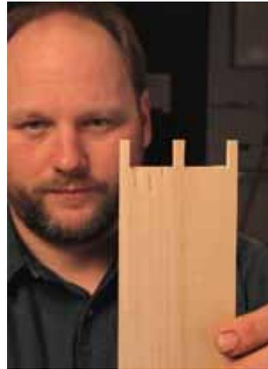
**3** When you finish making the template, here's what it should look like. For this 3"-wide drawer, I made two notches. Each of the teeth is 1/4" wide. You can make the notches almost any width you want. The spacing can be varied by using a smaller template guide in your router.
