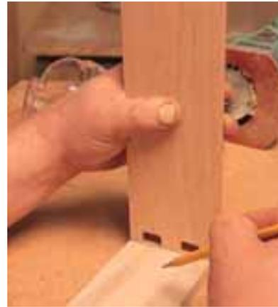
**5** Now lay out the tails by tracing around the inside of your pins. A sharp pencil is key.
